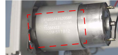
Figure 1-89. Reinstalling the CR Motor
