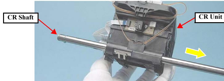
Figure 1-93. Removing the CR Unit (4)
