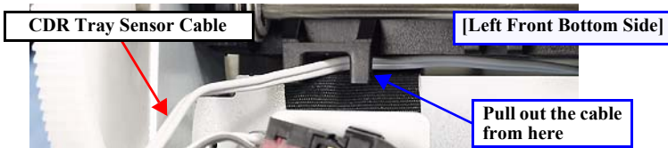
Figure 1-112. Routing the CDR Tray Sensor Cable
