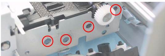
Figure 1-73. Reinstalling the Ink System (1)
