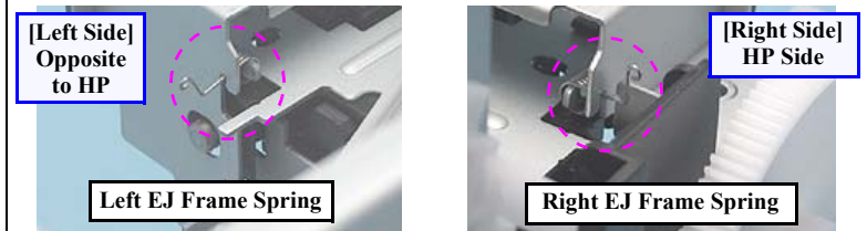
Figure 1-81. Reinstalling the Front Frame (2)
